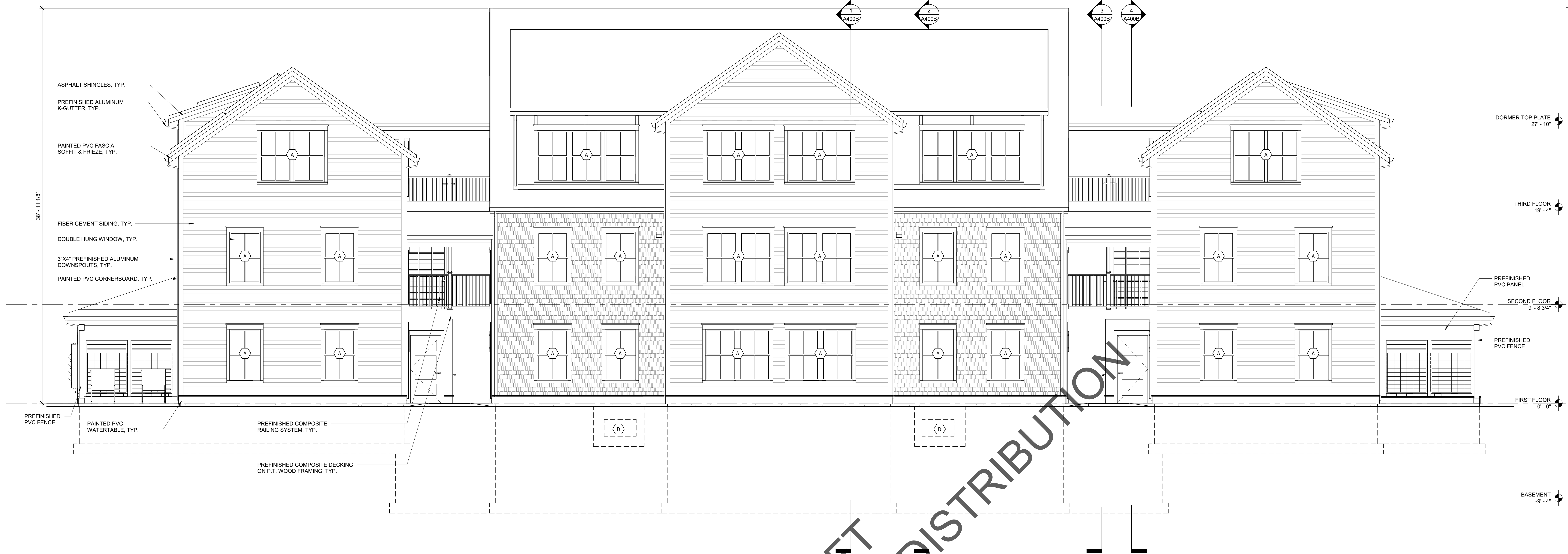
1 BUILDING TYPE B - NORTH ELEVATION 1/4" = 1'-0"
